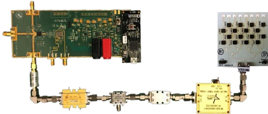
Achieves fast beam alignment: less than 1ms
