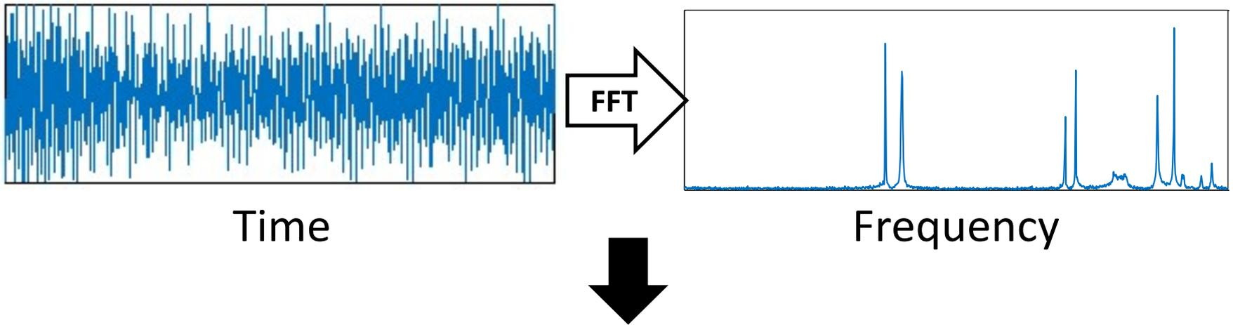
We leverage sparsity to compute the Fourier transform faster than FFT
