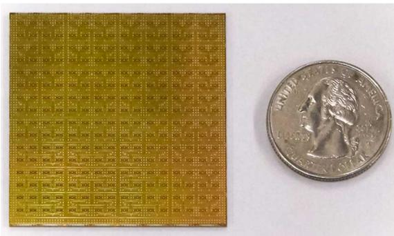
Small Wavelength enables thousands of antennas to be packed into small space
