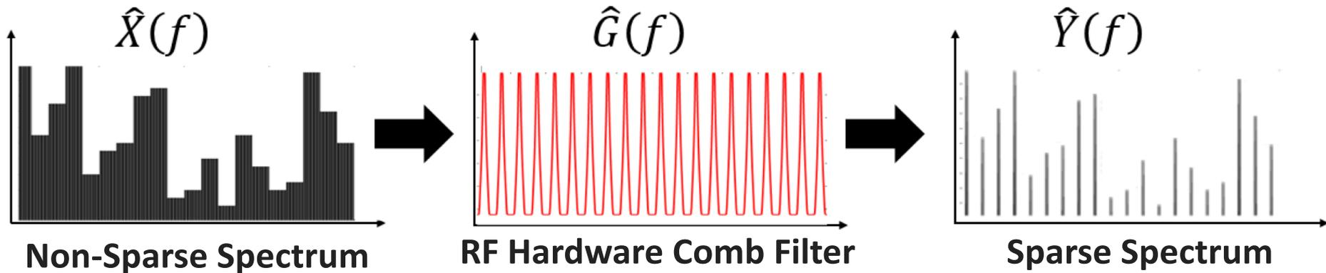
Using MEMS acoustic resonators
