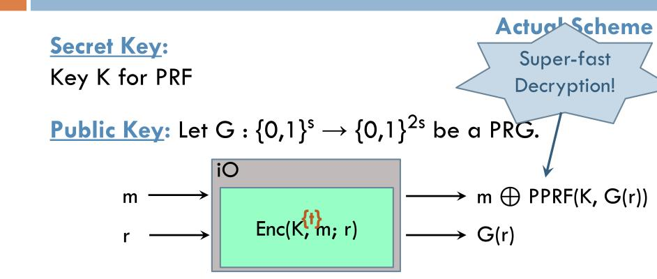
Challenge ciphertext: c\* = (t, m ⊕ PPRF(K, t)), t uniform in {0,1}<sup>2s</sup>.
