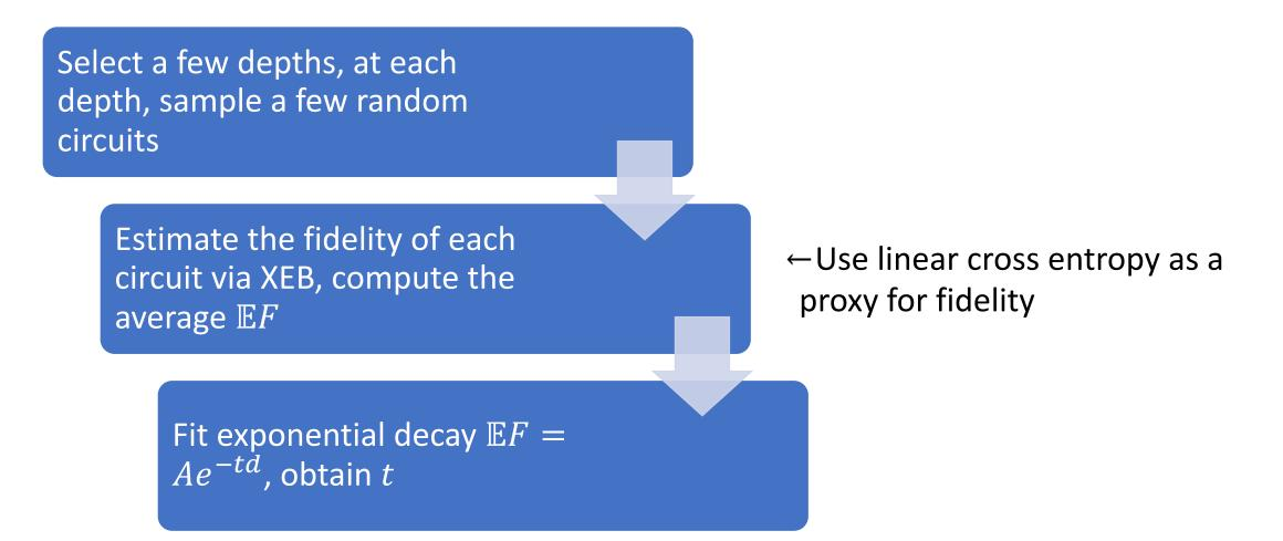
*t*: the effective noise rate on a layer of arbitrary two-qubit gates
