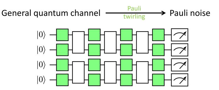
Can simplify the noise to a Pauli channel  $\{p_a\}, a \in \{I, X, Y, Z\}^n$  without changing the logic of the circuit
