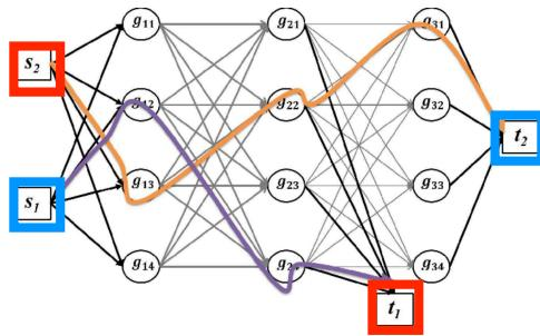
$$\begin{aligned} \max \quad & \sum_{p \in \mathcal{P}} f_p \\ \text{s.t.} \quad & \sum_{p: p \ni e} f_p \leq c(e) \quad \forall e \in E, \\ & f_p \geq 0 \quad \forall p \in \mathcal{P}. \end{aligned}$$
