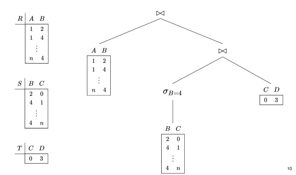
$R \bowtie (\sigma_{B=4}(S) \bowtie T)$  $\bowtie$  Ø R $A \quad B$  $\mathbf{2}$ 1 1 4  $\bowtie$ Ø AB4 n $\mathbf{2}$ 1 4 1  $B \quad C$ : SCB1 4 CD4  $\sigma_{B=4}$ n2 0 0 3 4 1 4 n4 nBC $\mathbf{2}$ 0 4 TCD1 3 0 4 11 n
